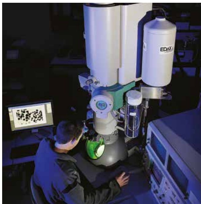
Transmission electron microscope in use at the Australian Microscopy and Microanalysis Research Facility (NCRIS network), University of Adelaide. This microscope is used to characterise a range of samples such as minerals, nanoparticles, ceramics, surface coatings and other materials for advanced manufacturing. Source: Australian Microscopy and Microanalysis Research Facility.
