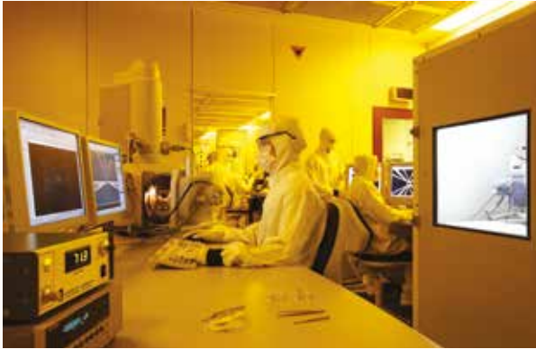
Electron-beam nano-patterning tools at the University of New South Wales node of the ANFF (NCRIS Network). This node manufactures Australian-made silicon quantum logic devices for quantum computing. Source: ANFF. Photo: Paul Henderson-Kelly.
