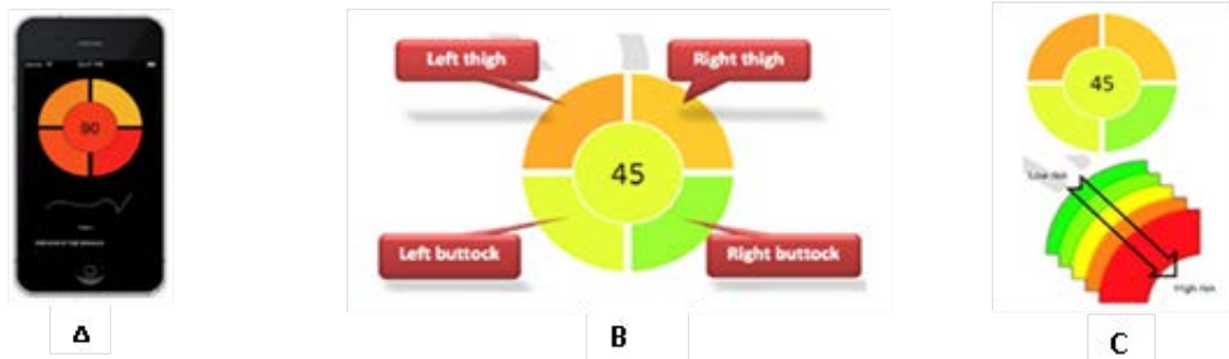
Figure 1. The iPod Touch provides the visual feedback (A). The middle number denotes the level of risk that the person has at that time (B). The higher the number, the higher the risk. This concept of graduated risk is depicted using an array of colours where green is low risk, yellow/orange is higher risk and red is the highest risk (C). The highest risk number is 99. It is based on a sophisticated algorithm based on duration of time sitting since last repositioning and the magnitude of the pressure of the buttocks on the mat.
