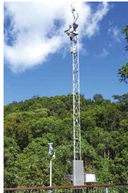
Flux tower in Queensland operated by the Terrestrial Ecosystem Research Network (NCRIS network) to measure the exchanges of carbon dioxide, water vapour, and energy between the biosphere and atmosphere. Source: Dr Cacilia Ewenz, Terrestrial Ecosystem Research Network.
