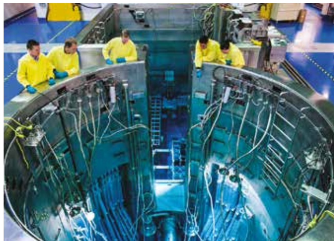
The OPAL Research Reactor is one of the world's most effective multi-purpose reactors. The high energy beta particles from spent nuclear fuel immersed in water give rise to the distinctive blue glow called Cherenkov radiation. The OPAL Research Reactor is used for nuclear medicine, scientific research and industrial applications. Source: Australian Nuclear Science and Technology Organisation.
