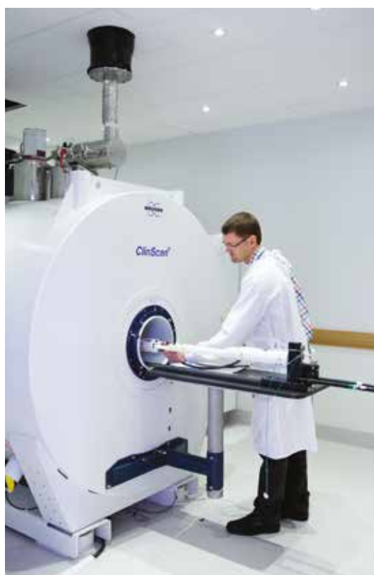
Preclinical combined MR-PET scanner within the University of Queensland node of the National Imaging Facility (NCRIS network) at the Centre for Advanced Imaging. This flagship instrument is unique, contributing to the development of innovation imaging in the fields of theranostics development, oncology, neurodegenerative disease and cardiac function. Source: National Imaging Facility.
