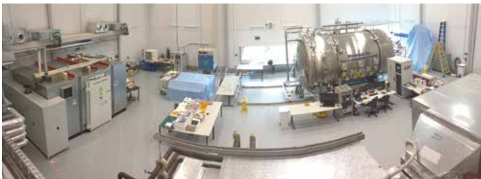
The 'Wombat XL' Space Simulation Facility in the Australian National University Advanced Instrumentation and Technology Centre, Mt Stromlo, creates space-like conditions to support designing, testing and constructing space industry components and cryogenic instruments. Source: Dr Naomi Mathers, Australian National University.
