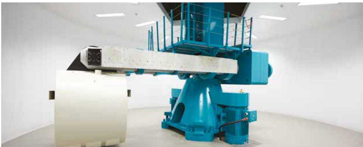
Ten metre centrifuge at the Indian Ocean Marine Research Centre at the University of Western Australia. The centrifuge is used for geotechnical modelling, marine research and to identify potential resources. Source: National Geotechnical Centrifuge Facility.
